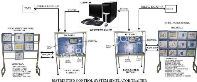
The **Distributed Control System Simulator Trainer (SAP - 90)** outlines the principle of Distributed control System used in Industrial Environment. The Static Application Panels provide an idea of different Process Plants. The Static Application Panels (SAPs) are mounted on M S Powder coated Frame and can be arranged in sequence as per the requirement.
